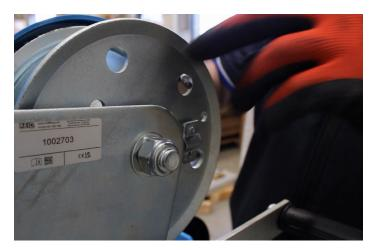
Feed the cable through the drum of the winch and terminate under the clamp, making sure not to fix on the fuse and tapered section.
