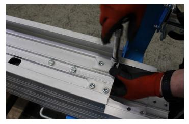
Fit the stops to the fixing plate in the designated holes at the bottom of each column.
