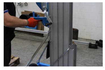
Move the loading wheel to the top position and secure the column sections with the column brake.
