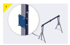
The following instructions detail the assembly of the PlusWinch bracket [RAWB010200] for the TDAVIT.
