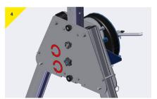
> Fully tighten both the top bolt and bottom pin. The winch bracket should sit flush with the plate.
