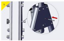
Insert the bolt into the top hole and secure using the knurled knob, leaving it loose so that the head sits proud of the plate.
