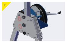
> Fully tighten both the top bolt and bottom pin. The winch bracket should sit flush with the plate.
