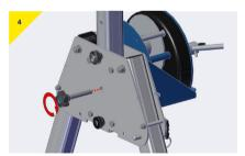
> Straighten the winch and insert the lower pin.
