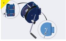
> Adjust the position by tightening the hex bolts.
