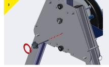
> Straighten the winch and insert the lower pin.
