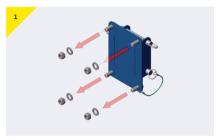
> Remove the washers and nyloc nuts from the bracket.
