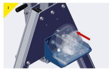
Hook the brakeet over the bolt head.
