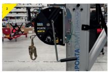
Insert the handle as shown into the free spool mechanism and anchor point.
