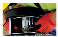
Wrap the cable tightly, ensuring 4 safety windings and place the end of the cable in the outer clamping location.
