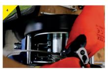
> Pull the cable tightly around the drum and tighten the inner bolt to secure the cable.
