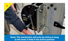
Retain the activation position and pull out as much cable as required.
