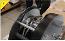
> Ensuring the winch drum remains static, wrap the wire rope tightly **4 times** around the drum.
