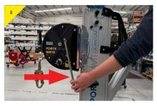
Pull the handle as shown to activate the freespool mechanism
