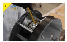
Ensure the wire rope is pulled tightly around the drum and tighten the inner bolt to secure the wire rope as shown.
