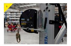
> Ensure the winch is secured to the lifting equipment.
