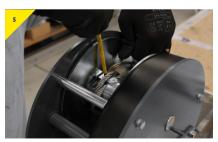
Secure the wire rope end by tightening the outer securing bolt.
