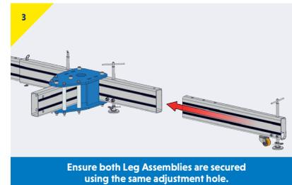
Ensure both Leg Assemblies are secured using the same adjustment hole.
