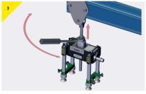
Engage the ratchet and apply the load. Once the required loading has been achieved, hold the load for the amount of time determined by the local authority regulations. De-load by rotating the ratchet in the opposite direction.
