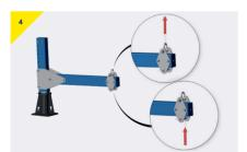
Depending on the device used for testing the socket, pull or push up the Test Davit using the necessary equipment to the required load. Once the Davit has been assembled in place it is ready for a device to be attached to the shackle point or clevis pin to begin the test.
