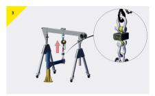
> Ensuring the loadcell reads 0 before starting. Apply load to the test davit using the chain block. Once the required loading has been achieved hold the load for the amount of time determined by the local authority regulations. De-load the test davit by reversing the chain block.
