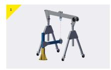
Position the PORTAGANTRY REPORT over the test davit ensuring the trolley sits directly above the shackle on the beam.
