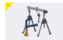
Fit the chain block and the loadcell in between the trolley on the gantry and the shackle on the test davit.
