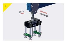
With the drop rod in its lowest position, place the device underneath the beam and secure using the supplied clevis pin and r-clip.
