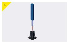
Insert the column into the socket.
